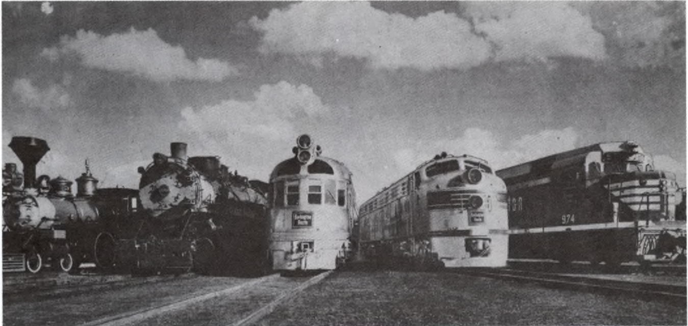
From Left: Diamond stack #35, typical of American-type wood and coal burners in use from 1850 to well into the 20th Century; Coal-burning 4960, Mikado-type build in 1923 for freight service; a Burlington Zephyr, first diesel-powered, stainless steel streamlined train in the world introduced in 1934; E-9 passenger built by Electro-Motive Division of General Motors; and Turbocharged, GP-35 locomotive built in December, 1963 by Electro Motive. (Burlington RR photo)
